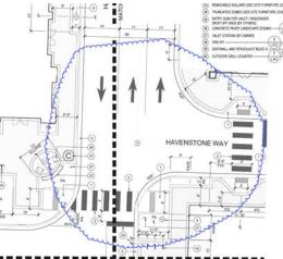
6. Include the lane configuration striping for truck turning exhibit. This is to ensure the turn ends up in appropriate lane.
