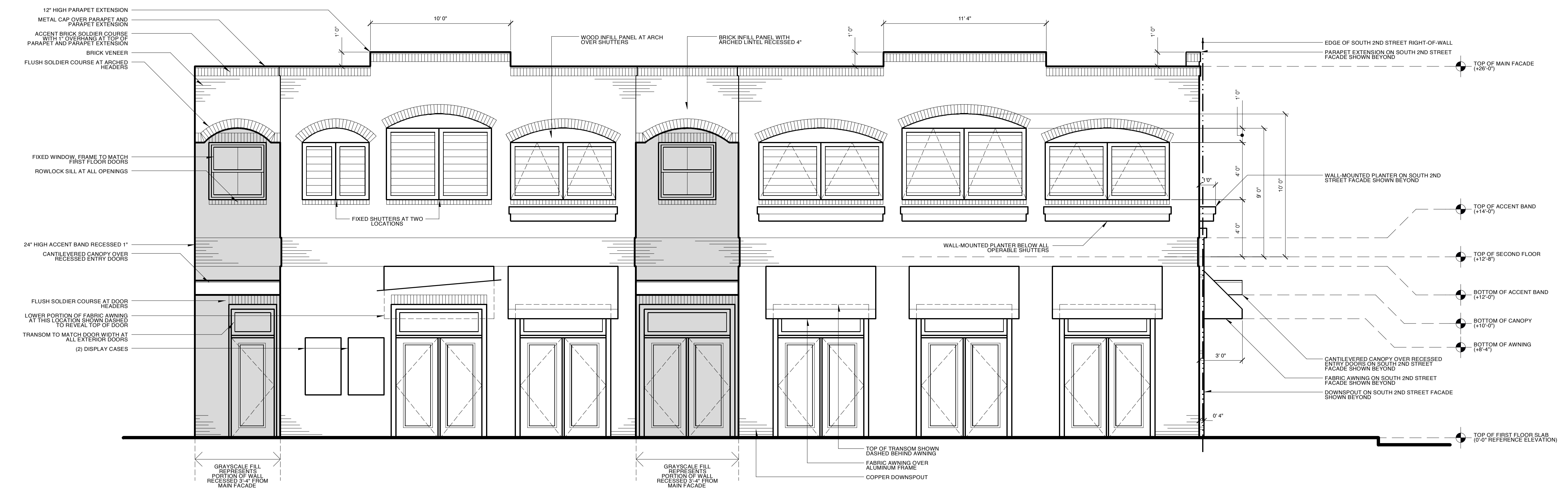
1/A5 • Market Street Exterior Elevation Scale: 1/4" = 1'-0"
