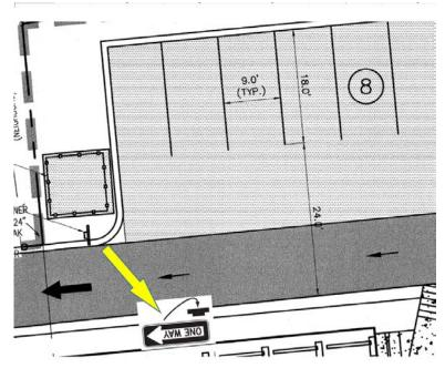
The backing stub is to be 10' deep by 15' wide. Please dimension. [Chapter VII ,Detail SD 15-12 CofWTSSM]
