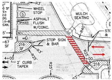
2. City's 20'x70' sight distance triangle is shown at the driveway accessing Sir Tyler Dr. Please revise the sight distance triangle as per the proposed new ROW on the plans. [Sec.18-529(c)(3)CofW LDC] Add a note indicating that all proposed vegetation within sight triangles shall not interfere with clear visual sight lines from 30"-10'. [Sec.18-556 CofW LDC]
