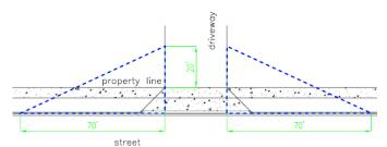
7. The Darlington Oaks shown at the driveway must have be positioned and maintained in a manner that will not interfere with clear visual sight lines from 30" to 10'.
